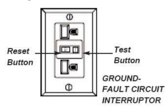
If you do have G.F.C.I.'s, it is recommended that you test (and reset) them monthly. When you push the test button, the reset button should pop out, shutting off the circuit. If it doesn't, the breaker is not working properly. If you don't test them once a month, the breakers have a tendency to stick and may not protect you when needed.
